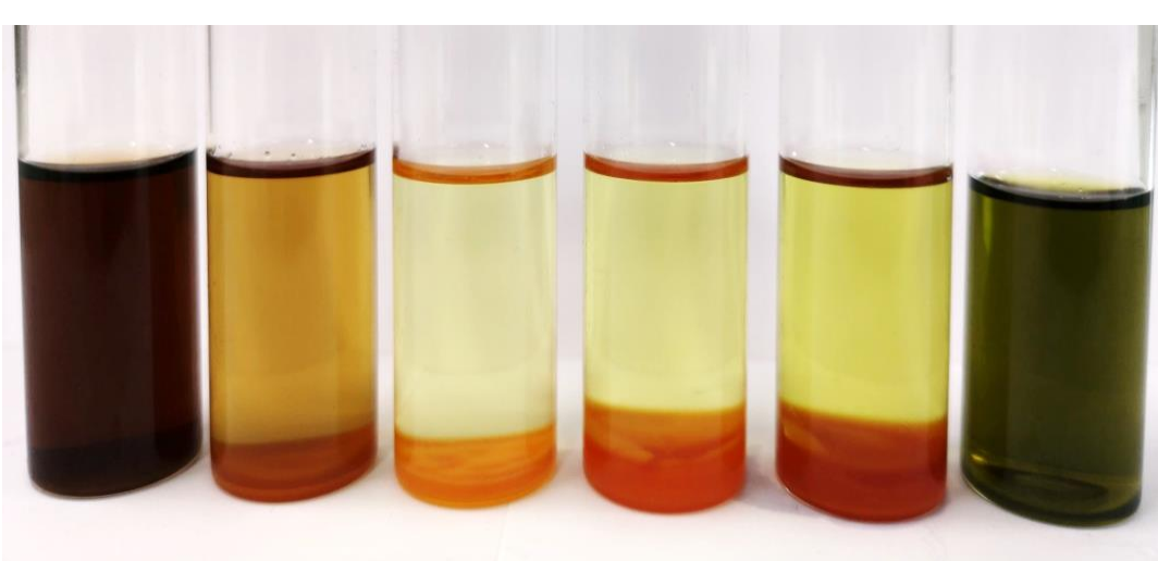
Fe – rich sludge dissolved in DESs
