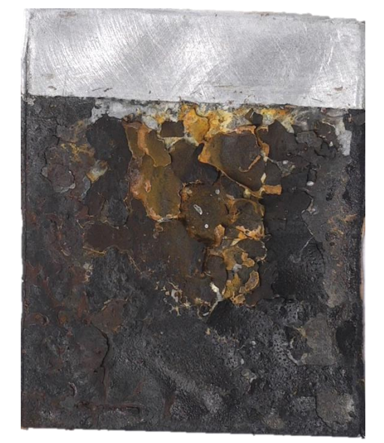
Cementation of Fe out of DES on Zn substrate
